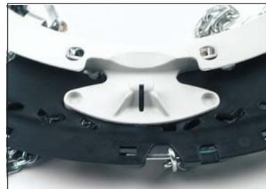
Now move the grey safety ring clockwise, as long as both buttons are locked.
